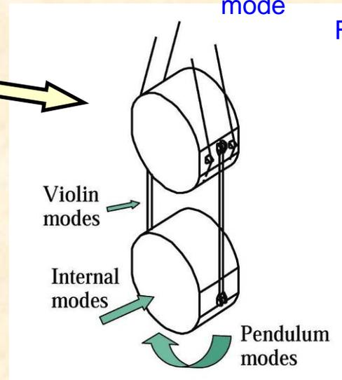
Ultra-low mechanical loss suspension at the heart of the interferometer
