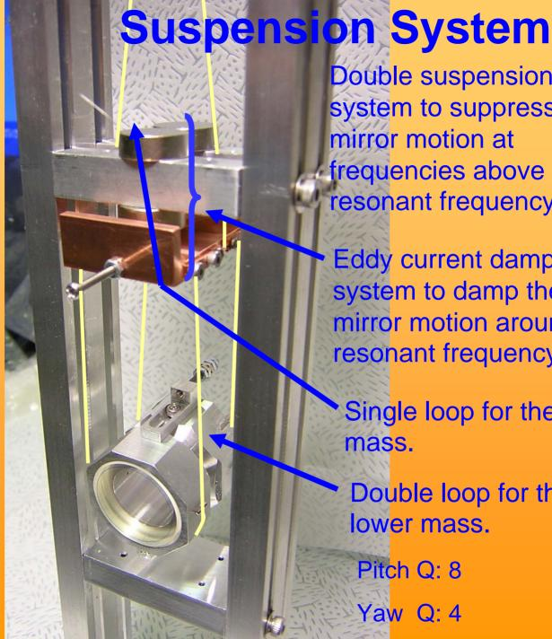
**Double suspension** system to suppress the mirror motion at frequencies above the resonant frequency.
