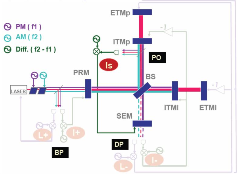
L+, L- by single modulation & demodulation (arms) lp,ls,l- by double modulation & demodulation (central part)
