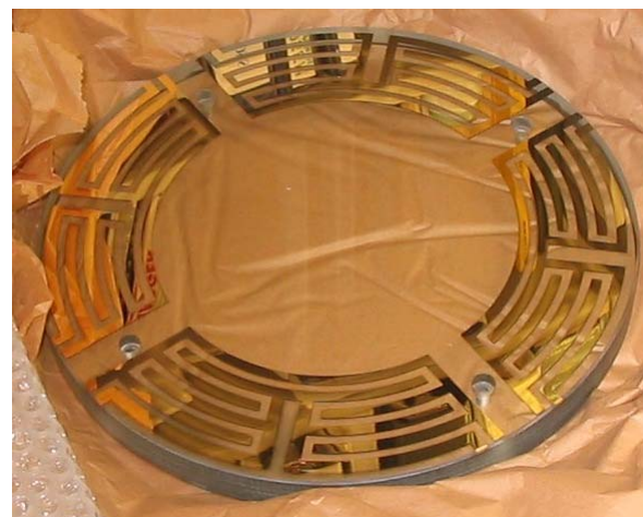
Prototype gold-coated face-plate for electrostatic actuation
