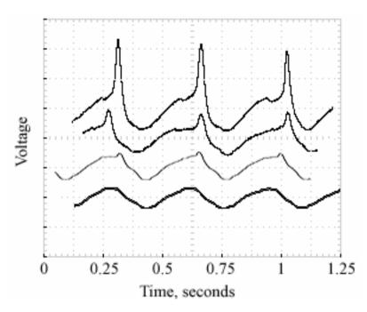
Relaxation of distribution of charge deposited by local contact electrification on fused silica sample: pictures from oscilloscope at different time
