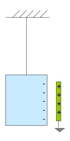
• Variation of electrical charge  $\Delta q$  produces variation of force  $\Delta F$ :
