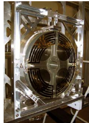
Electrostatic drive gold coating shown for reaction mass of controls prototype
