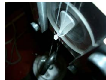
12 kg long term load test on bonded ear
