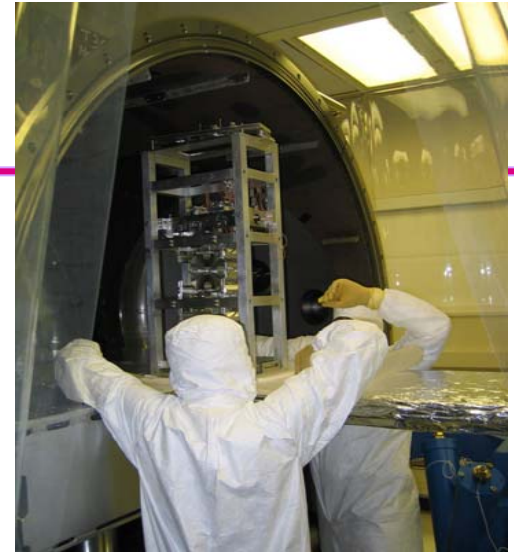
'Controls' Triple Installation at LASTI
