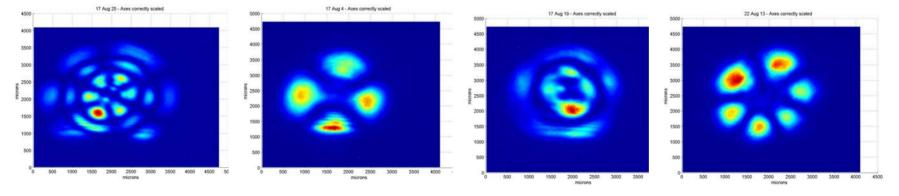
Diffraction around beam baffle eliminated
