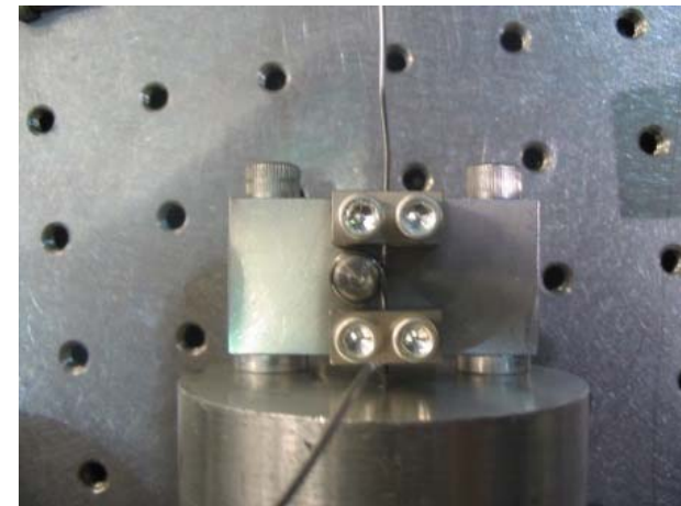
Simplified clamp used for testing revised design
