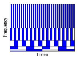
The decomposition provides high time resolution at high frequency (low scale), and low time resolution at low frequency (high scale). Example of S3 glitches:
