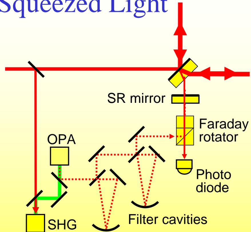
Reflecting squeezed light at two subsequent filter cavities provide the desired frequency dependence in the generic case (for fixed angle homodyne detection).
