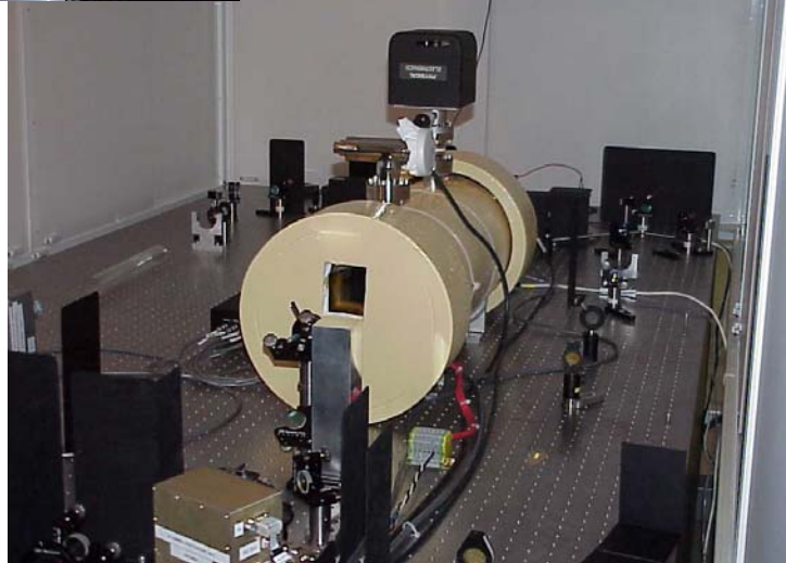
Stabilization cavities for laser beam— Widely used for precision optical applications
