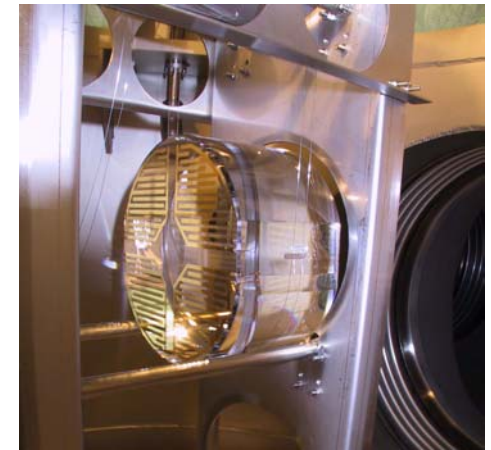
Reaction mass with gold plated grid for electrostatic control
