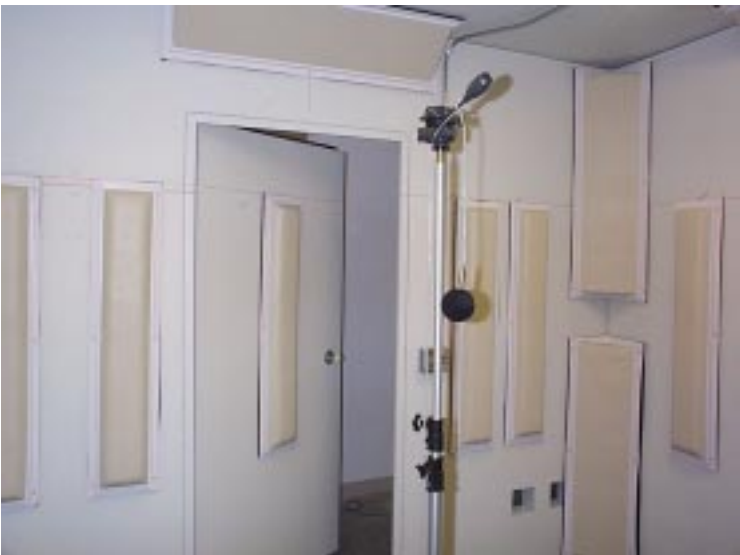
Enclosure: attenuation factor of about 10 at low f ; with absorption kit, 20 to 30
