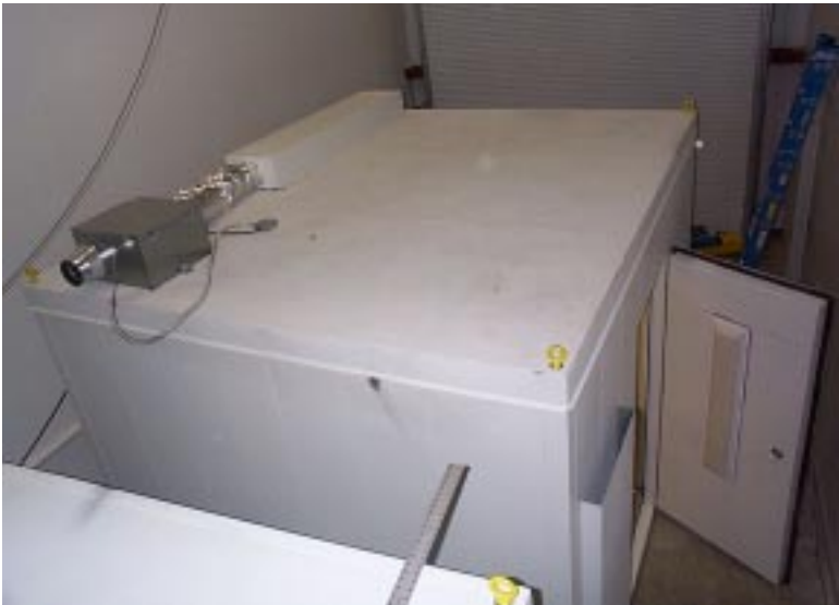
Enclosure: attenuation factor of about 10 at low f ; with absorption kit, 20 to 30
