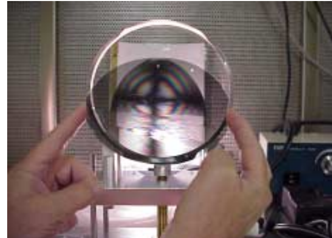
C - axis sapphire from Crystal Systems Inc, with visible flaw Q > 1.7 \times 10^8 (Willems et al)
