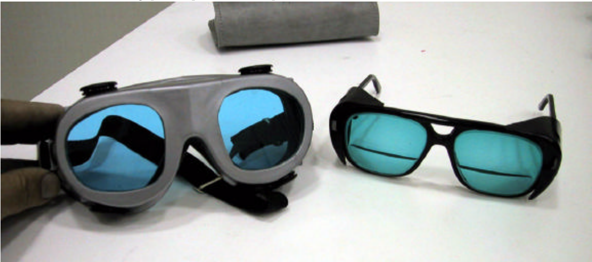
These 2 types provide protection from a direct beam
