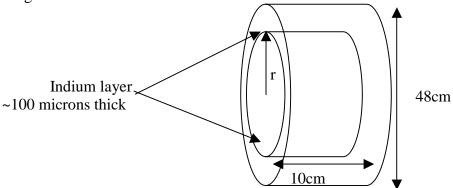
Imagine joining inner mass to outer silica donut by a thin layer of indium (or indium/tin).
