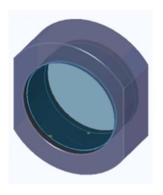
Complete or circumferentially segmented indium layer between the Cradle and the fused silica optic
