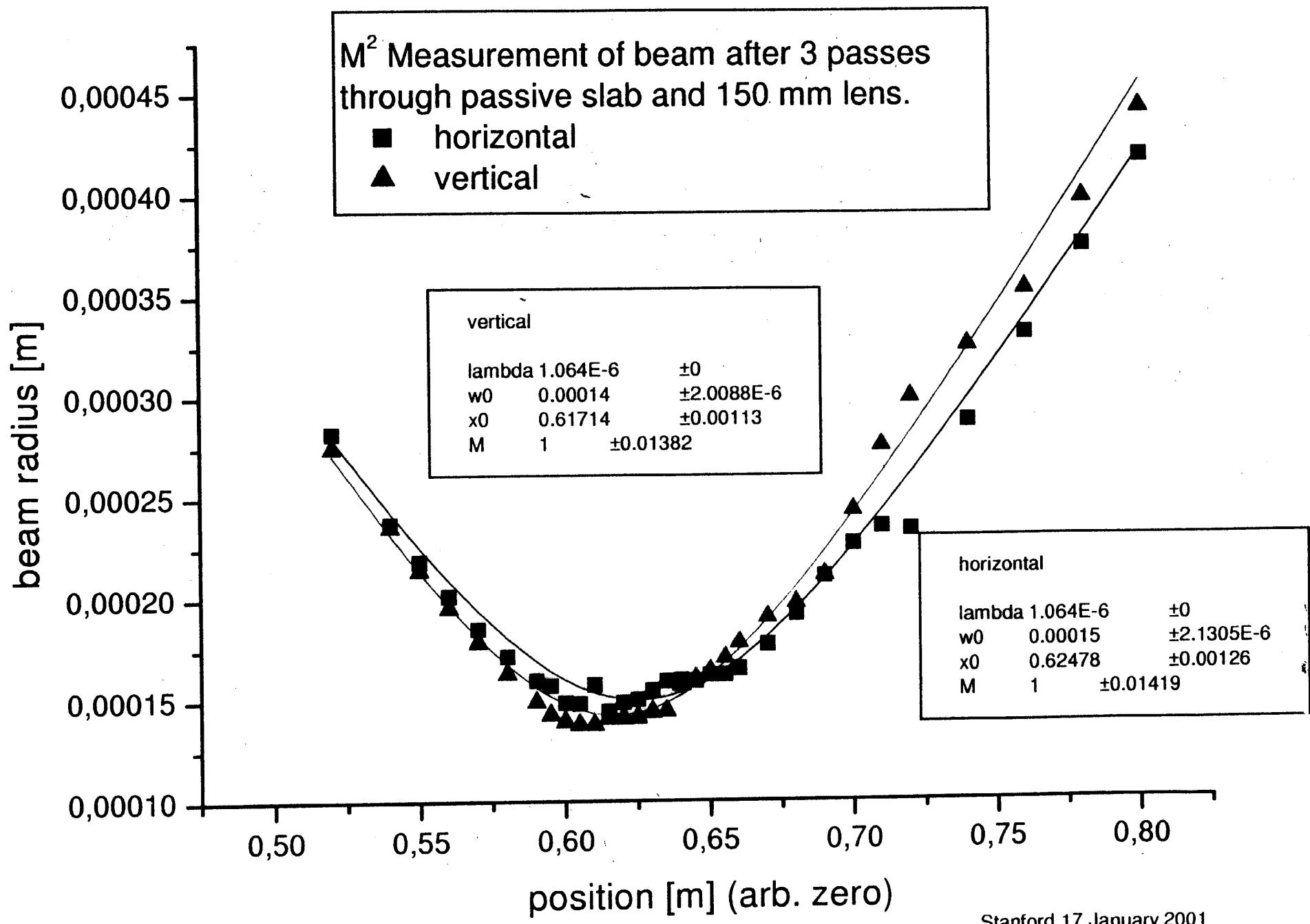
$M^2$  measurement after hot slab
