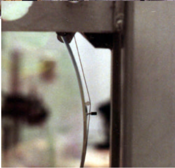
test mass is balanced on 1/100 th inch diameter wire to 1/100 th degree of arc
