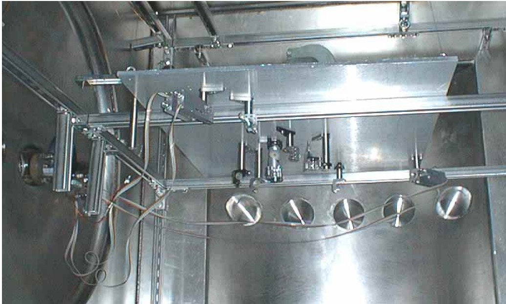
The suspended table in the vacuum system holds most of the components of the interferometer
