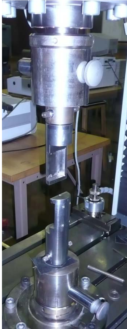
Figure 2.1 Shear strength testing set-up
