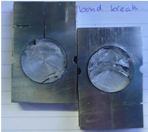
Figure 3.3 Disc MP2 broken at ~ 5 MPa
