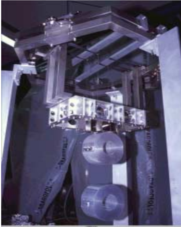
Initial assembly of triple pendulum
