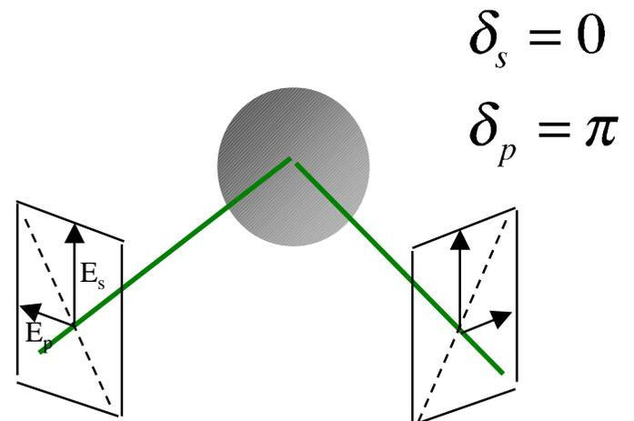
A dielectric mirror can introduce a phase shift between the s and p polarization components of a beam, thereby rotating the polarization
