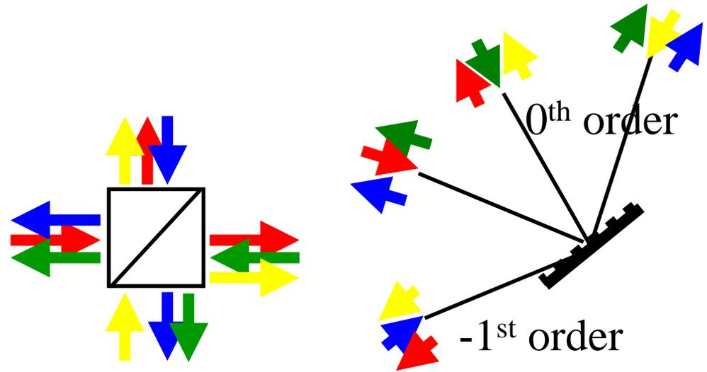
A grating has the undesirable effect of converting laser frequency noise to pointing noise and distorting the spatial profile of the diffracted beam. These effects can be compensated for:
