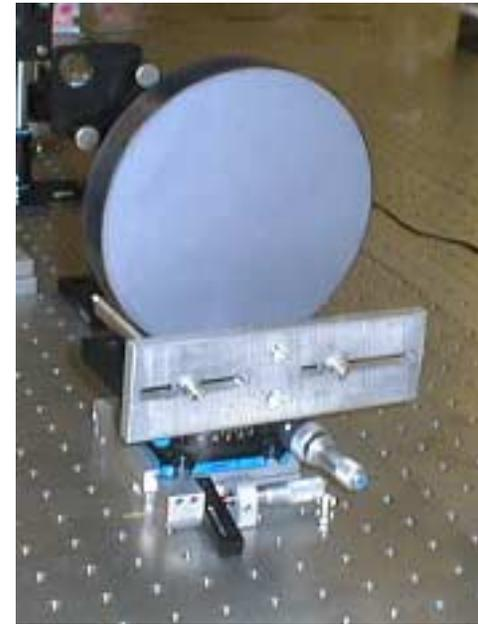
6 inch diameter (1 inch thick) silicon substrates, coated and polished cost \$7,000 from General Optics. Only 15% more than fused silica
