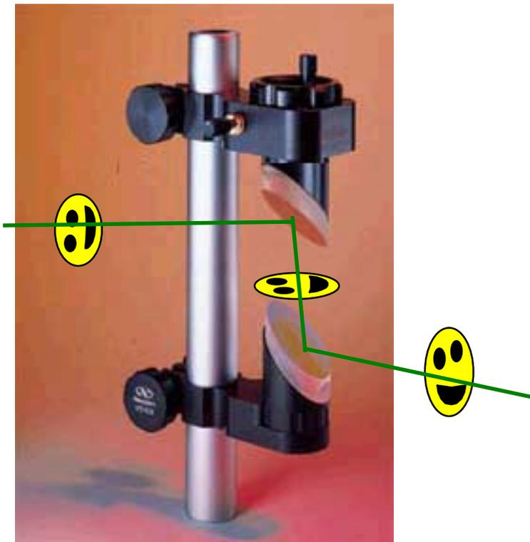
A periscope can rotate the spatial profile of a beam, thereby rotating the polarization
