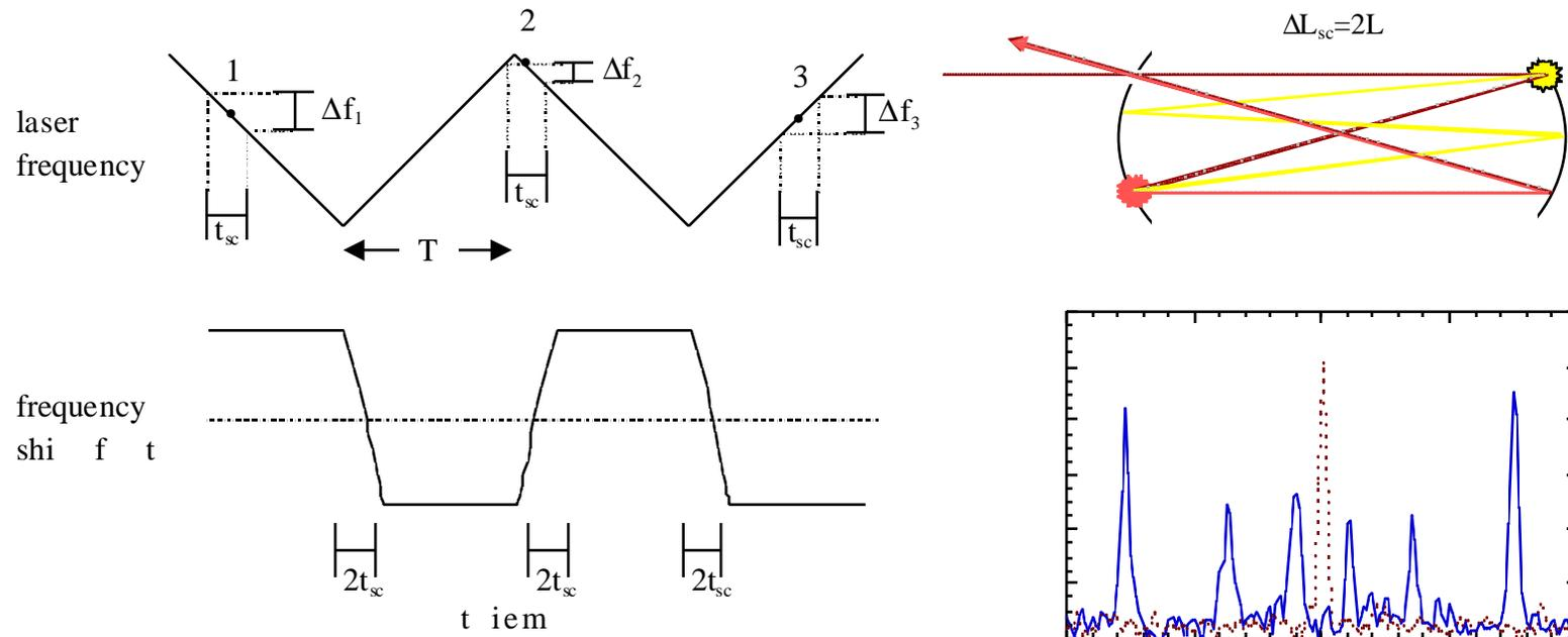
Any noise from scattered light with a delay,  $t_{sc}$ , much less than the modulation period,  $T$ , will be shifted
