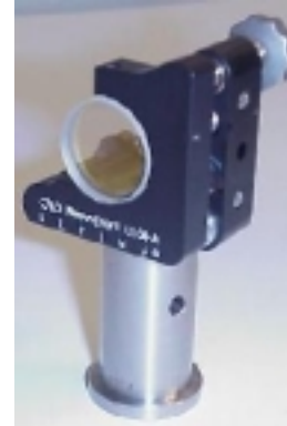
Newport Ultima 100 (“open”) with 1” post -580 Hz
