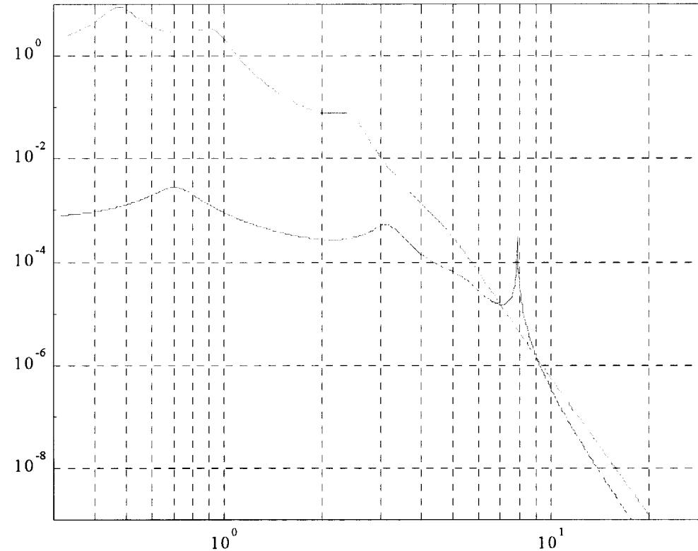
Longitudinal (red) and vertical (blue) isolation curves with local controls on, incl. cross-coupling of 0.001 in vertical. Overall length 1.7 m.
