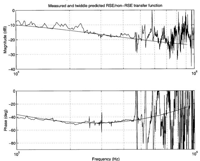
>>Somewhat simplified optics - 60% PRM, 37% SEM. Arm cavity finesse of 300 (cavity pole roughly 200 kHz).
