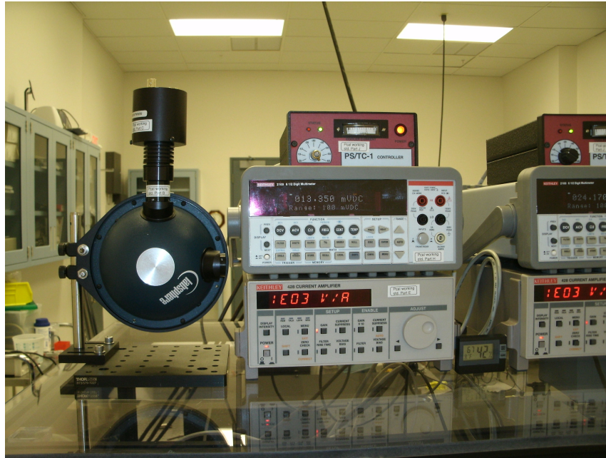
Figure 27 – eLIGO Working Standard power sensor including the integrating sphere, photo-receiver module, fast current amplifier, digital multimeter, and power supply/thermo-electric cooler controller.
