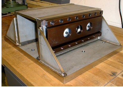
Figure 3: flexure and spring seats installed (pre-compression spring side)
