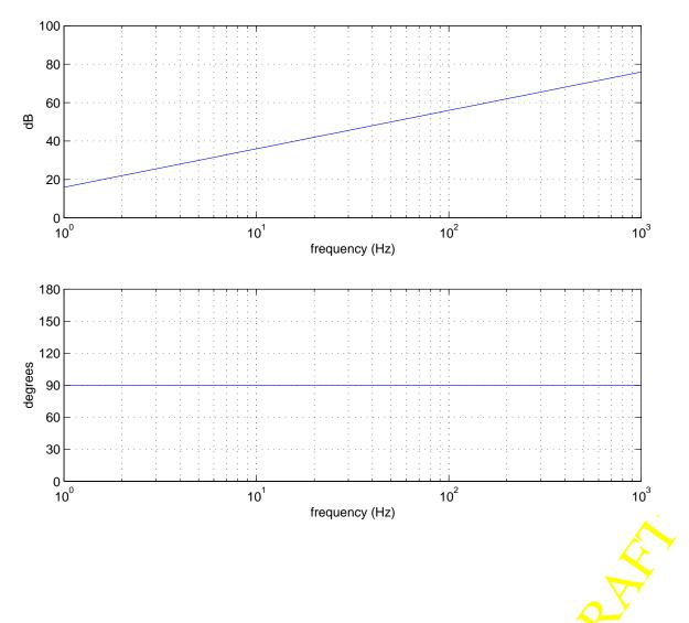
Therefore, the digital filter representation of the phase modulation effect of a Pockels cell driven by a time dependent voltage is  $A/2\pi \cdot DF[s]$ , where DF[s], the digital filter, is a zero at DC and a regulator pole at high frequency, if required.
