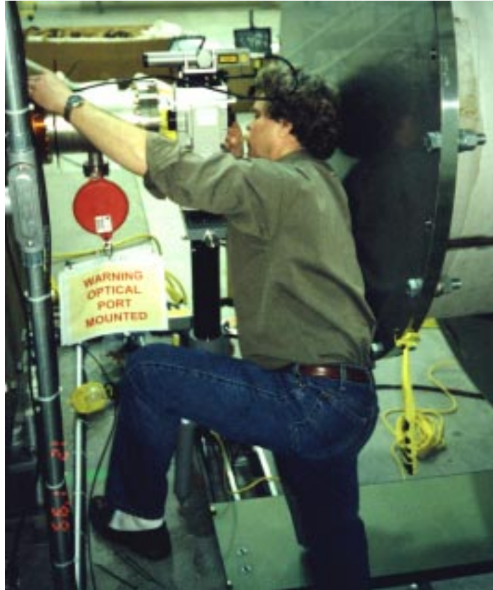
Figure 2: Theodolite mounted on tripod stand between cryopump and Y1 beam tube end cap viewport in Hanford LVEA. Operator is John Worden of LHO.
