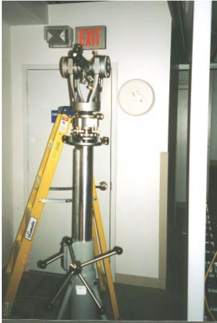
Figure 3: Optical transit square set up in line with IAM-6, -9 and -12 for reading out monument offsets.
