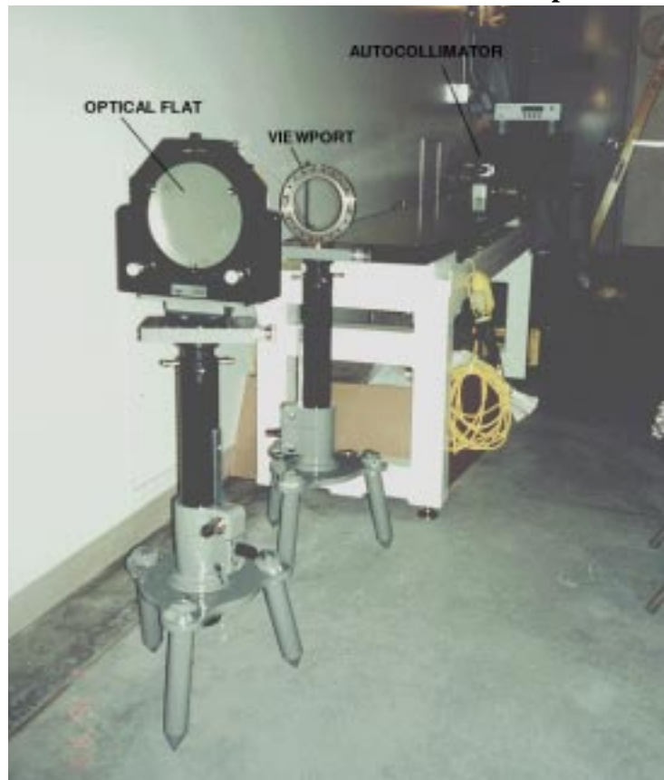
Figure 5: Setup for measuring the transmissive angular deviation of the viewport after removal from the beam tube endcap.
