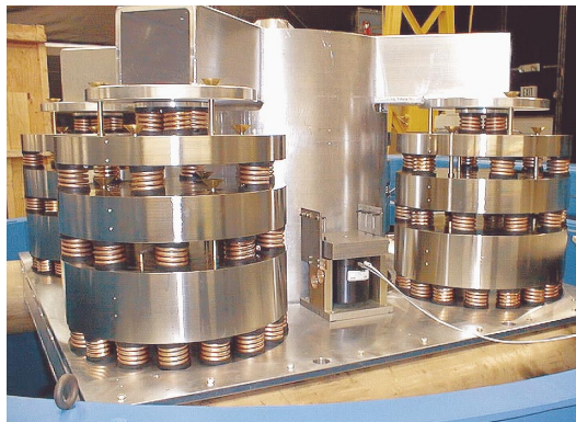
Figure 5: prototype stack with reaction mass shakers in position on the support platform.
