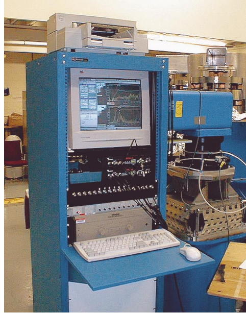
Figure 7: the PC-based SigLab 20-42 data acquisition system.
