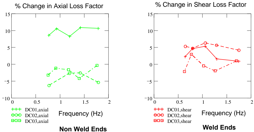
Figure 4: Percent change in axial and shear loss factor from non weld coil to weld coil.
