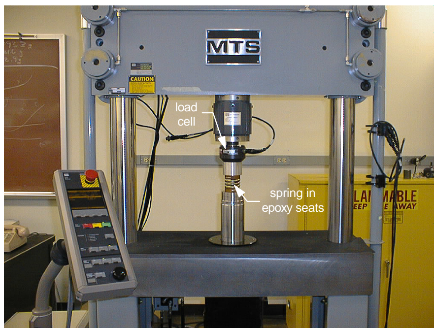
Figure 3: Static and fatigue test setup.
