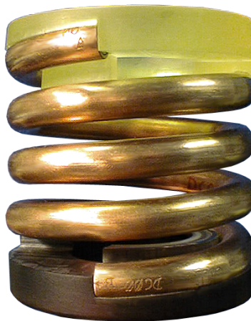
Figure 8: Damped coil pre-prototype DC00 in its molded epoxy seats.
