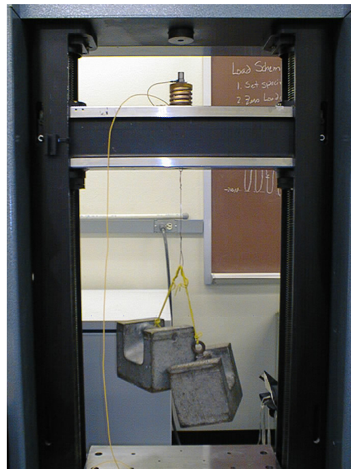
Figure 14: Modified free decay test setup for evaluation of axial loss factor; threaded rod replaced with cable to eliminate parasitic bending mode.
