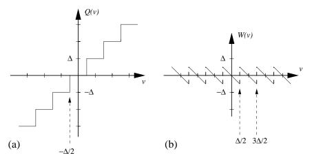
FIG. 2. (a) The quantization function Q(v) which maps the analog signal into integer multiples of  $\Delta$ , the quantization level, by rounding. (b) The error function which is defined as W(v) = Q(v) - v.
