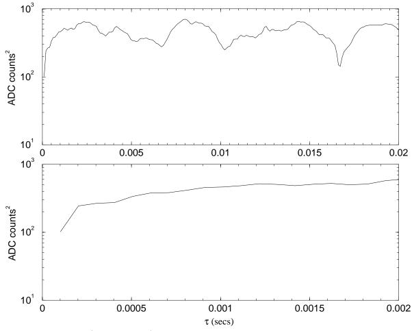
FIG. 3. The function  $f(\tau) = \langle (v(t) - v(t+\tau)^2 \rangle$  in units of (ADC counts)<sup>2</sup> for a quiet stretch of data from the prototype 40m interferometer. The lower graph is zoomed in by a factor of 10 on the upper graph. It is clear that the condition in Eq. (3.6), with  $\Delta = 1.0$  is well satisfied even at for  $\tau = (2f_N)^{-1} \approx 10^{-4} \,\mathrm{sec}$ .
