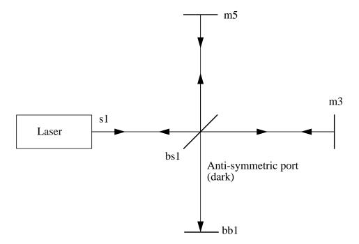
We've had to add a "beam dump" at the antisymmetric port, which is simply an end mirror with 0 reflectivity, which allows us to make a connection to the beamsplitter from the antisymmet-
