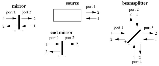
From the commands in the *ifo* file specifying the interferometer construction, *Twiddle* constructs a matrix which, when inverted and multiplied by the appropriate source vector, gives the electric fields at each component in the interferometer,
