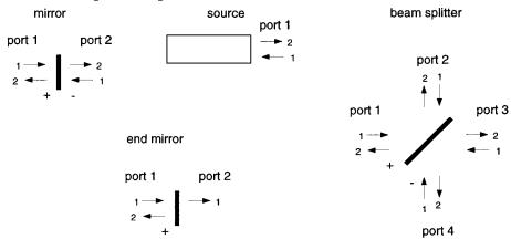
From the commands in the *ifo* file specifying the interferometer construction, *Twiddle* constructs a matrix which when inverted and multiplied by the appropriate source vector gives the electric fields at each component in the interferometer.
