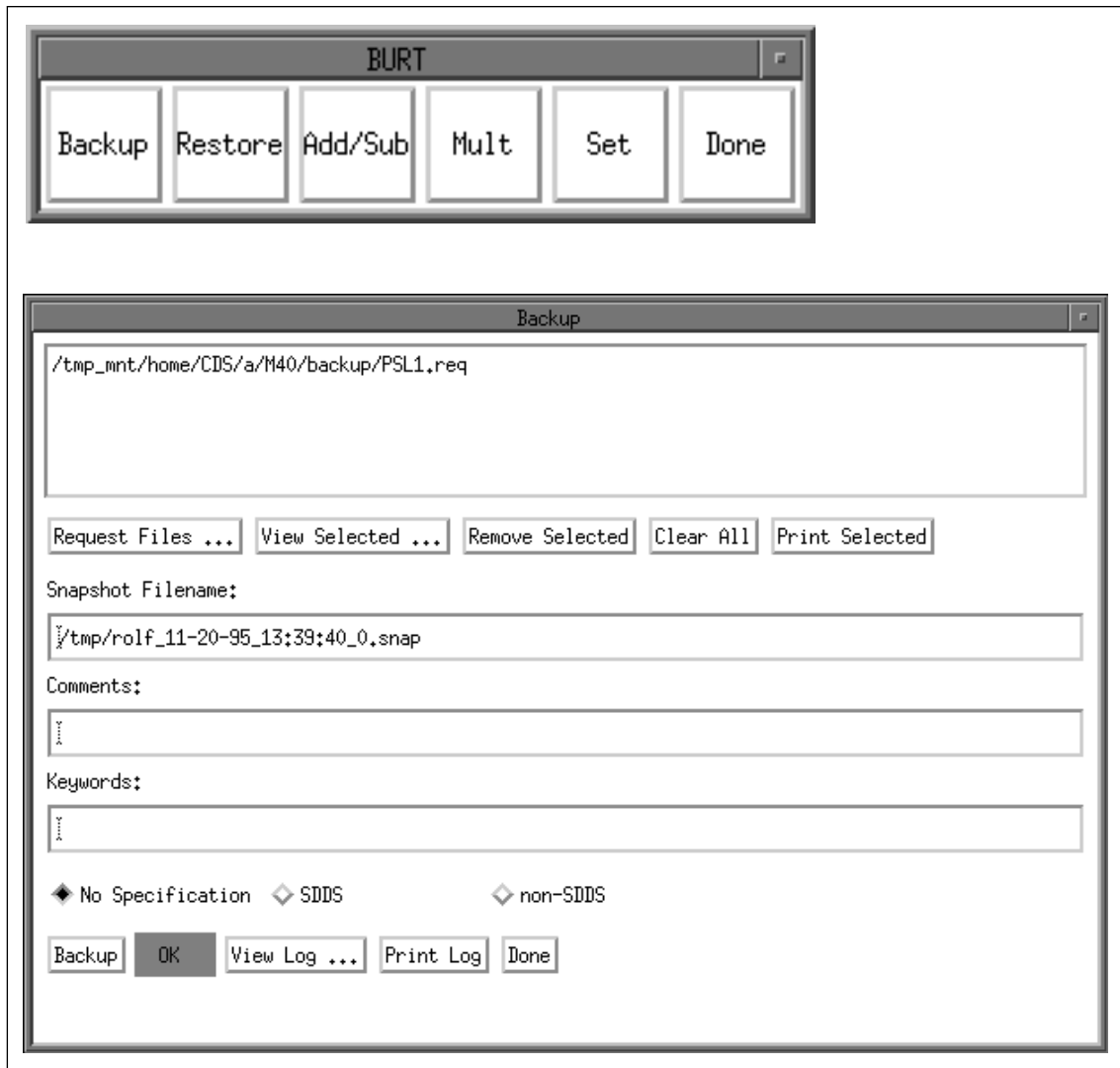
Figure 31: Backup and Restore Tool (BURT)
