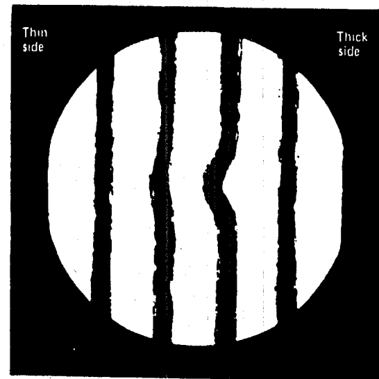
Figure 1.18. Kink formation in the straight Fizeau fringes of a slightly wedged plate, obtained by locally heating the plate. The kink is pointing toward the thin side of the wedge.
