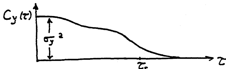
Fig. 5.3 Example of a correlation function that becomes negligible for delay times \tau larger than some relaxation time \tau_r .
