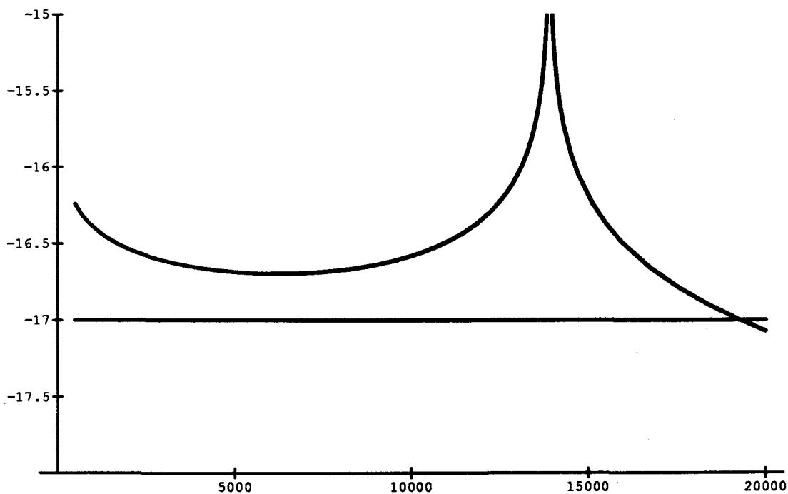
Figure 7 Plot of thermal noise in second lowest order mode \log_{10} (\text{cm}/\sqrt{\text{Hz}}) vs. frequency (Hz) for \phi(\omega) = 10^{-5} . The horizontal line shows the predicted sensitivity of 10^{-17} \text{ cm}/\sqrt{\text{Hz}} .
