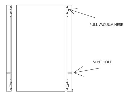
This solution allows the use of light disks because, although the holding force would still be of the order of 1000 N, the force is localized to the periphery, the lids are not subject to pressure over the entire surface and there is no need to make them very stiff.
