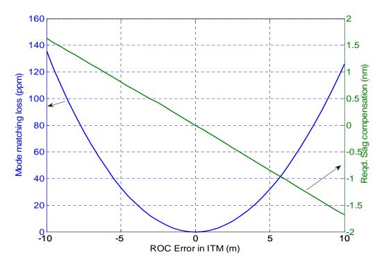
Fig. 7: Mode-matching error as a result of ITM ROC error. The green curve plotted on right y-axis shows the required compensation in terms of sag at the CP while the blue curve shows the residual mode matching loss after optimal compensation has been applied.
