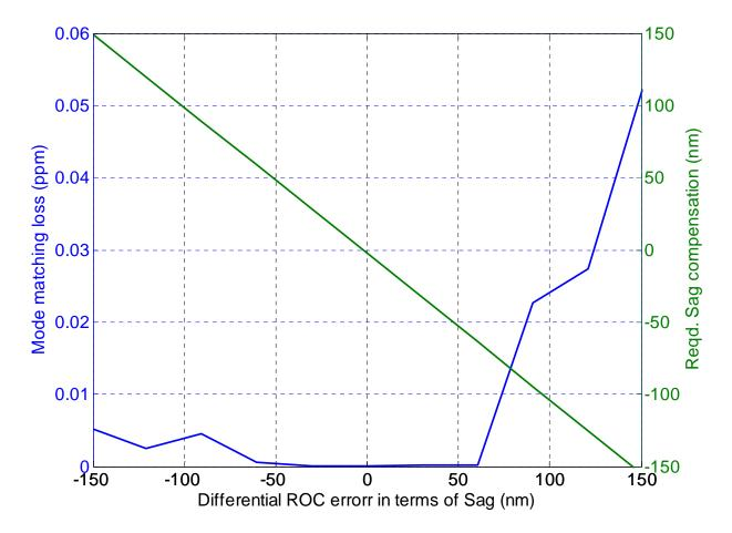
Fig. 6: Error compensation using CP for combined ROC differential errors in Michelson cavity. The x-axis values are the sag corresponding to a ROC error value in the cavity with 5.5 cm beam size. Plotted on left y-axis is the residual mode matching loss if we apply compensation at the CP according to the green curve plotted against right y-axis.
