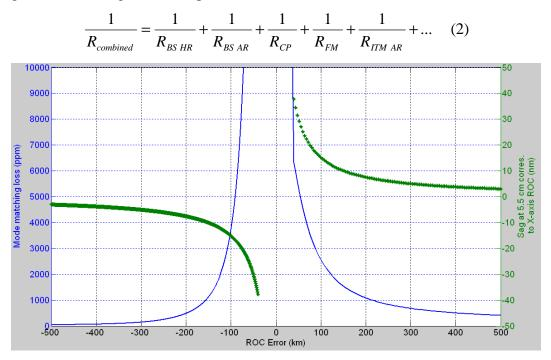
Fig. 4: Mode matching loss due to combined ROC error as defined in Eq. 2 plotted in blue against left y-axis. The corresponding sag (for a 5.5 cm beam) values are plotted in green on right y-axis.
