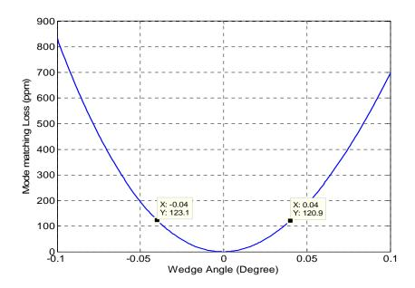
Fig. 2: Mode matching loss due to BS Wedge angle in SRC
