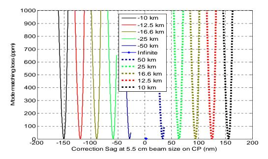
Fig. 5: Compensation of combined differential ROC error in the Michelson arm by operating on CP.
