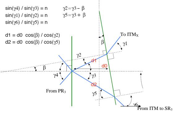
Fig. 1: Geometry of the BS wedge angle.
