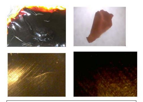
Above: Clockwise from upper left: Normal magnification, 10x magnification, 200x magnification, 60x magnification. While the sample appears very smooth to the naked eye, there are ridges visible at 60x and higher. These may have been produced in removing the sample from its aluminum tray.
