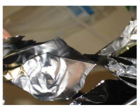
The above samples were created using PI-2525 and the heating profile above. The sample depicted in the two photos on the right was dissolved in T-9039 thinner, and the sample on the left was not. Both samples peel away from the aluminum tray smoothly and without breaking.
