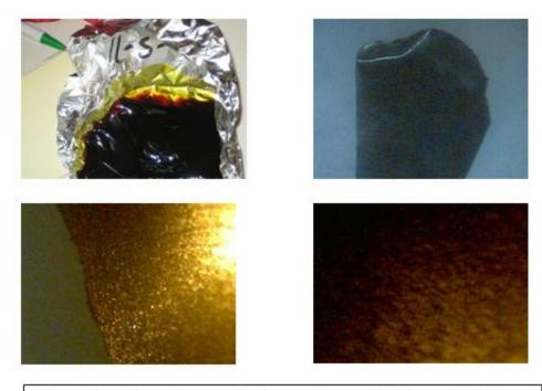
Above: Top Row—the sample at normal magnification and at 10x. Bottom—the sample at 60x magnification. The sample is very smooth, there do not seem to be any deficits—ompared to the second sample.
