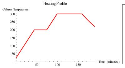
The initial heating profile used for resin PI-2525
