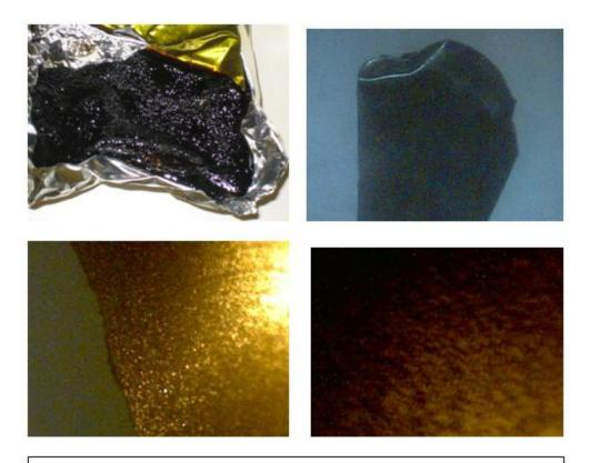
Above: Clockwise from upper left: Normal magnification, 10x magnification, 200x magnification, 60x magnification. Bubbling can be clearly seen, but there is no powdering, and the surface is fairly smooth even at high magnification.
