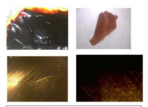
Above: Clockwise from upper left: Normal magnification, 10x magnification, 200x magnification, 60x magnification. While the sample appears very smooth to the naked eye, there are ridges visible at 60x and higher. These may have been produced in removing the sample from its aluminum tray.
