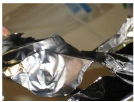
The above samples were created using PI-2525 and the heating profile of the figure above. The sample depicted in the two photos on the right was dissolved in T-9039 thinner, and the sample on the left was not. Both samples peel away from the aluminum tray smoothly and without breaking.
