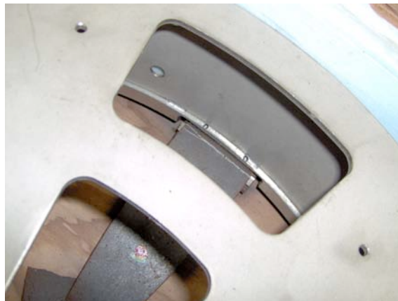
Figure 3, filter (TAMA model) with parts of blades laying at the bottom of the crate and close-ups of the broken blades.
