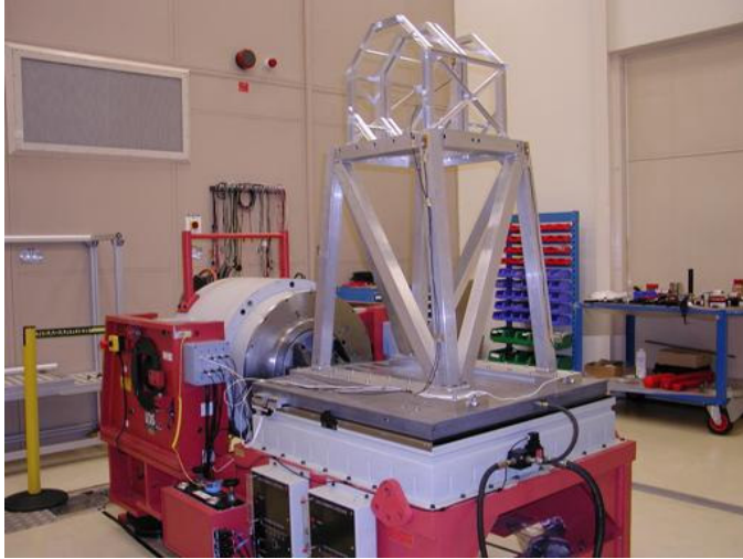
Fig 10. The LDS electro-dynamic shaker with sleeve and face plate design. (x axis test configuration)
