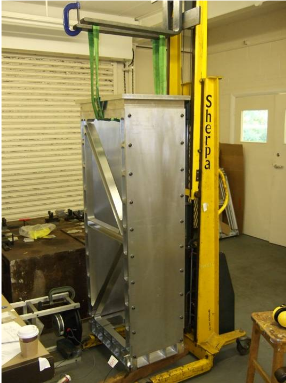
Fig 6. Beam splitter structure with shear plates suspended by a sling.
