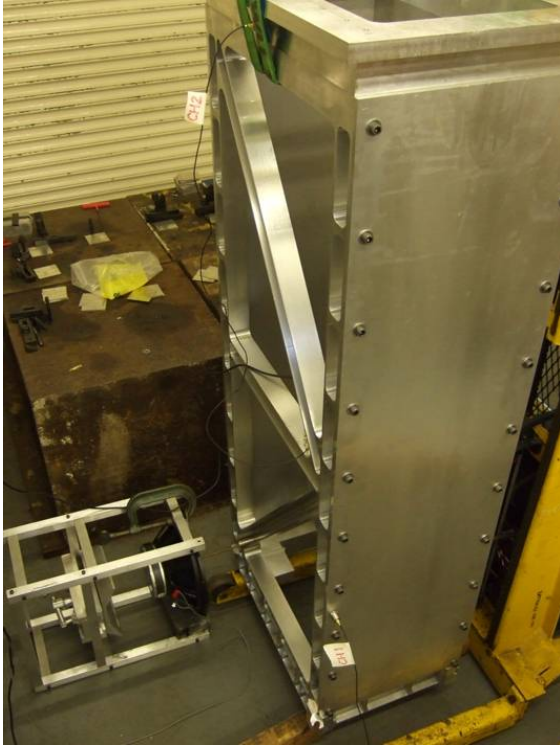
Fig 10. An accelerometer is positioned, in the middle of the top ring (top of the picture) representing channel two, and on the shear plate (bottom of the picture) representing channel one.
