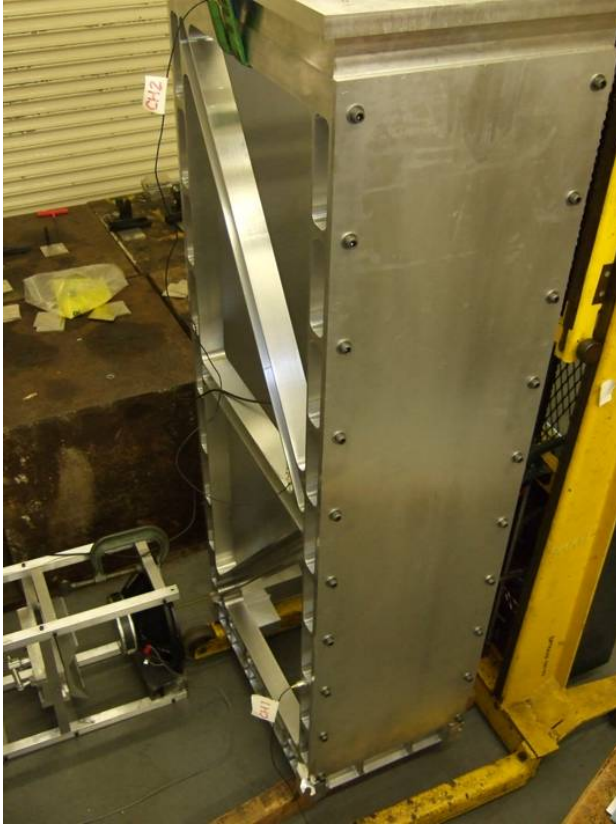
Fig 12. An accelerometer is positioned, in the middle of the top ring (top of the picture) representing channel two, and on the face plate (bottom of the picture) representing channel one.
