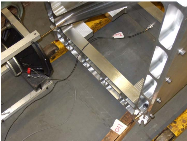
Fig 7. An accelerometer is positioned, in the middle of the bottom ring (top right of picture) representing channel two, and on the right hand side of the ring (bottom right of picture) representing channel one.
