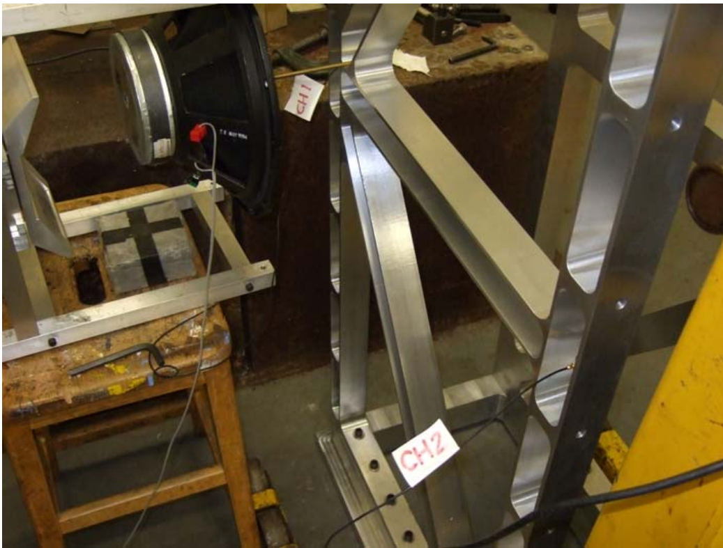
Fig 11. An accelerometer is positioned at the middle left hand side of the face plate (top of the picture), and at the middle right hand side of the face plate (bottom of the picture).
