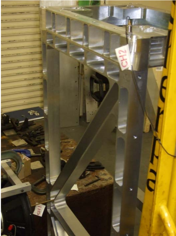
Fig 9. Accelerometers are positioned at the middle left hand side of the face plate, in the direction of the beam (bottom left in the picture), representing channel one, and at the top right hand side of the ring, normal to the beam (top right of the picture), representing channel two.
