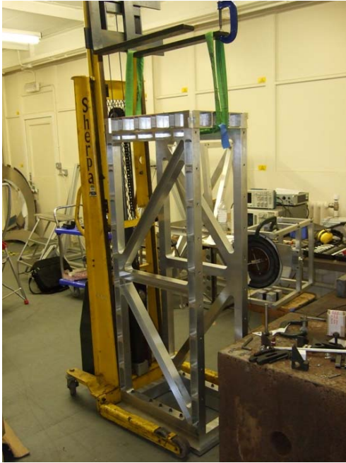
Fig 8. Beam splitter structure suspended at its end ring by at a sling.
