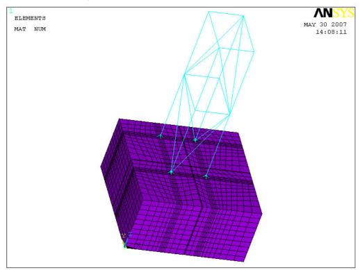
To get a good fix to the steel blocks, I added "extra feet" thus, at each corner. The spacing of these extra feet was set by the APDL parameter "fixoff" at 30mm from the base of the leg – simulating a fixation that spreads over about 60mm.
