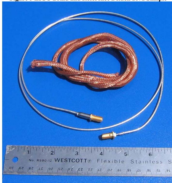
Figure 5 LIGO Braid and Reference Belden 1671 Sample
