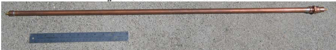
Figure 2 One Meter Triaxial Test Fixture
