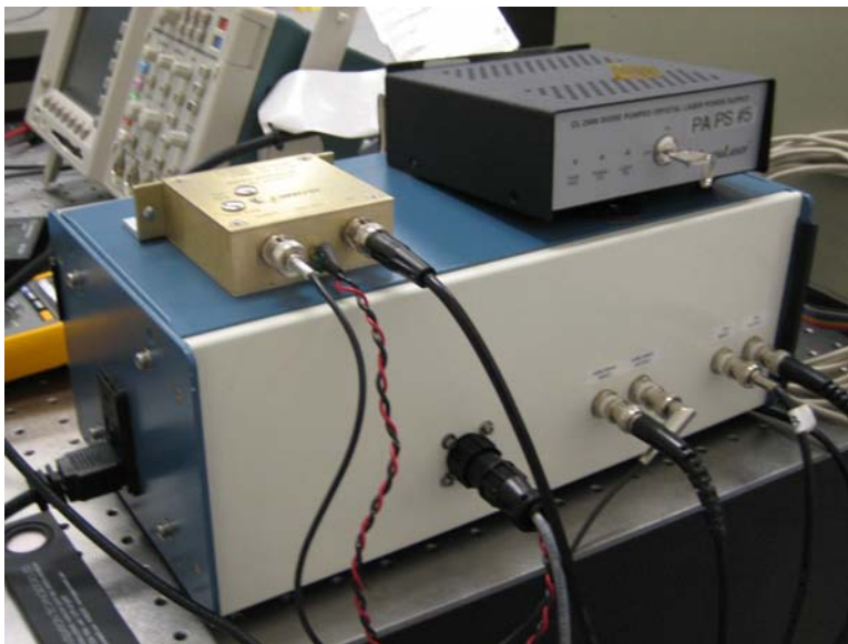
Figure 1 Pcal electronics modules. The large white and blue box houses the signal conditioning amplifiers. The AOM driver is gold box on top at the left. It uses the lower box for heat sinking. The laser power supply is on top on the right.
