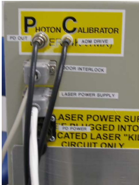
Figure 2 Pcal electrical feed-throughs in the upgraded configuration. The internal power sensor output utilizes the isolated BNC bulkhead connector on the upper left. The AOM drive input utilizes the isolated SMA feed-through on the upper right. The door interlock (two wires only) and the laser power supply to head interface are via 9-pin D connectors. The power for the internal PD utilizes the 4-pin CPC connector at the bottom. This would not be required with the proposed power sensor upgrade, which utilizes a photodetector operating in photovoltaic mode, if the current amplifier is mounted externally.
